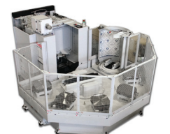
Vertical Pallet Pool
